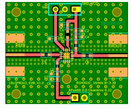
\*Dielectric constant  $\_$  3.38 \*RF pattern width 0.85T \*16mil thick RO4003PCB
