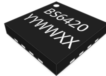
3mm x 3mm x 0.75mm, 16-Lead TQFN Package
